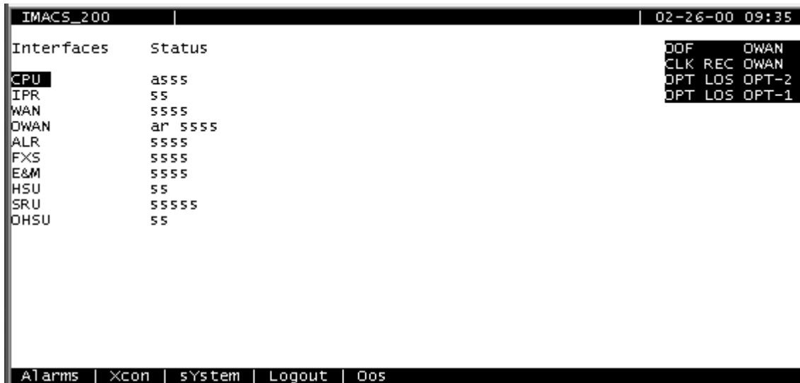
Figure 4-1. Main CPU level upon login
