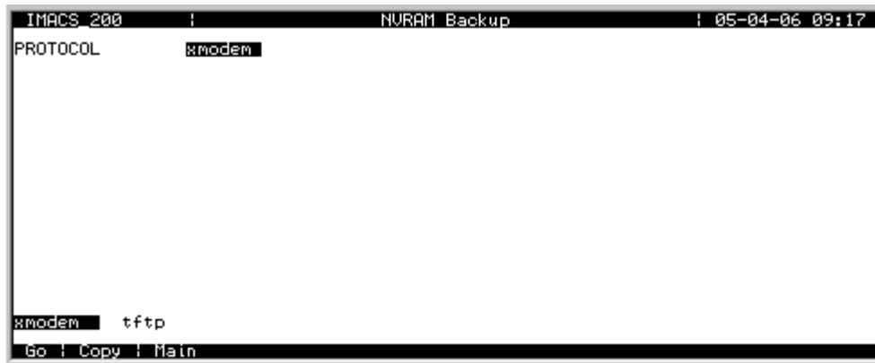
Figure 3-14.Backup (and restore) File Transfer Protocols
